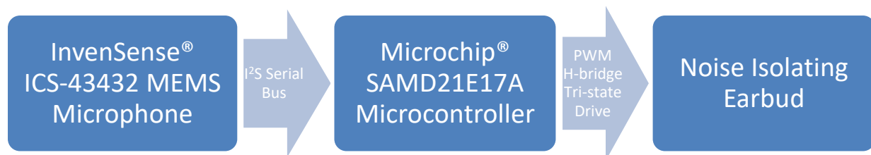
FIGURE 1: SIMPLIFIED HEARING AID DEMO HARDWARE DESIGN BLOCK DIAGRAM
